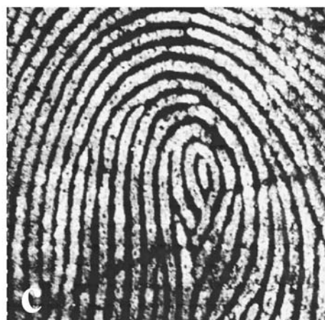
FIG. 4—Ethyl cyanoacrylate fumed mark on glass slide: (a) White light photograph of ethyl cyanoacrylate fumed fingerprint on glass slide. (b) Infrared spectrum of fingerprint ridge showing peak area at 1743\text{ cm}^{-1} used to generate image. (c) Monochrome representation of infrared chemical image.
